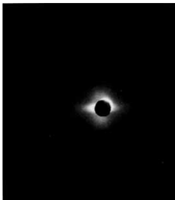
Figure 10 SAXS photograph of a partially stabilized 2% MA precursor fiber showing the two-point pattern along the meridian.
